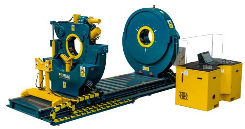
Forum Energy Technologies' AMC fully rotational torque (RT) bucking machine is a self-contained, free-standing, hydraulically powered unit designed for fast and accurate makeup and breakout of premium and non-premium threaded tubular equipment. The machine can handle up to a maximum torque of 200,000 ft-lb tracking thread, and run in from as low as 200 ft-lb.
